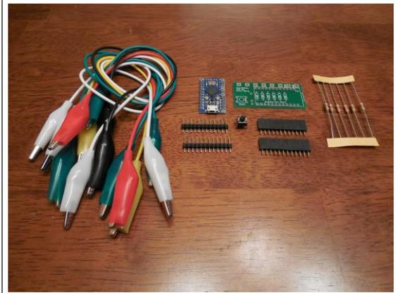
Cut an alligator clip off of one end on each wire.
