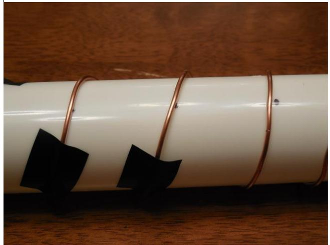
After the wire is aligned with all the dots, wrap tape around the wire to secure it to the tube.
