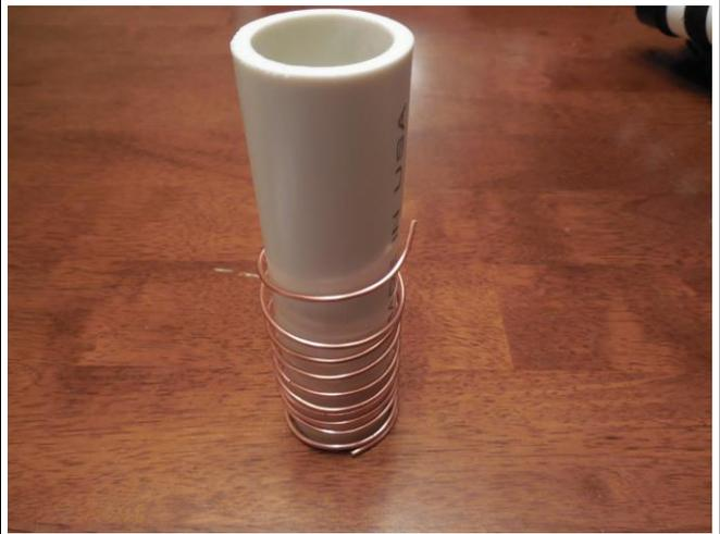
Align the copper wire along the dots you placed on the tube in a previous step. Use small pieces of tape to keep the wire in place.
